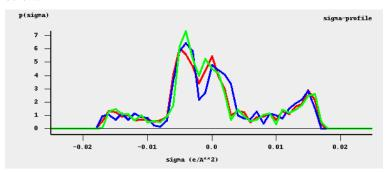
$\sigma$ -profiles of methanol (picture made with the CRS-GUI). In this picture the blue line is the  $\sigma$ -profile with the Esurf type of construction, the red line is that with the Delley type of construction with many surface points. For comparison, the green line is the  $\sigma$ -profile of methanol if a large QZ4P basis set is used, again with the Delley type of construction with many surface points.
