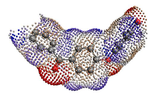
Fig. 5.2: Fig. 2. COSMO surface of the isolated Polyether ether ketone (PEEK) monomer.
